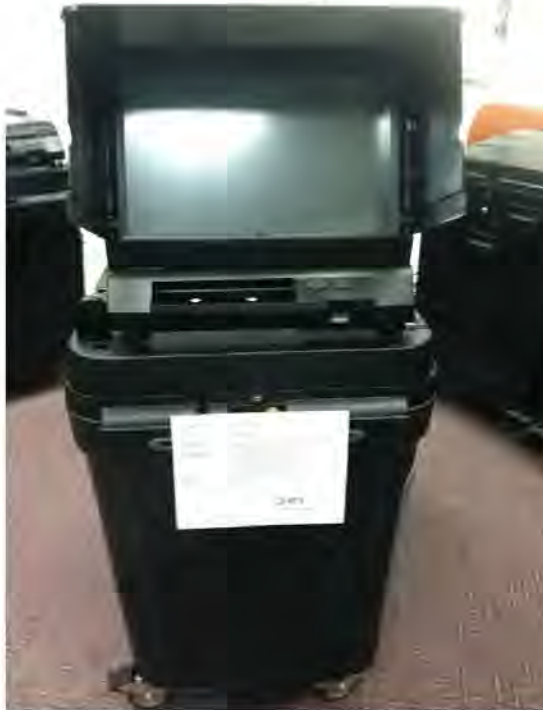
Figure 1-1: ImageCast Evolution (ICE) on Plastic Ballot Box
