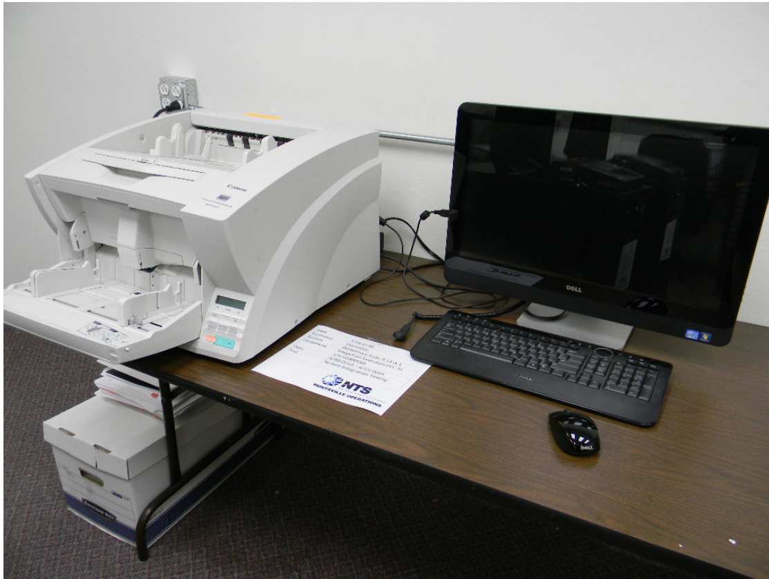
Photograph 3 System Integration Test: ImageCast Central
