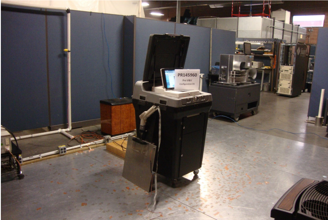
Electrostatic Discharge Test Setup
