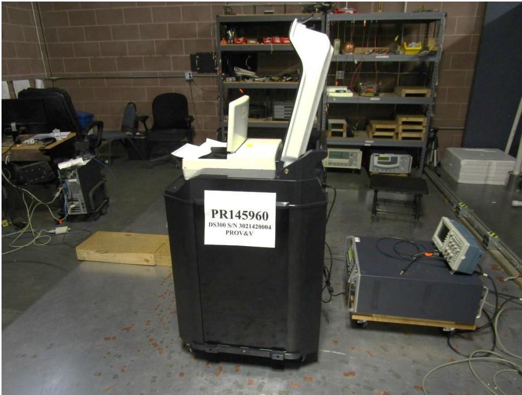
Electrical Fast Transient Test Setup
