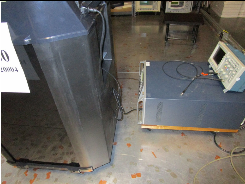
Electrical Fast Transient Test Setup – AC Mains
