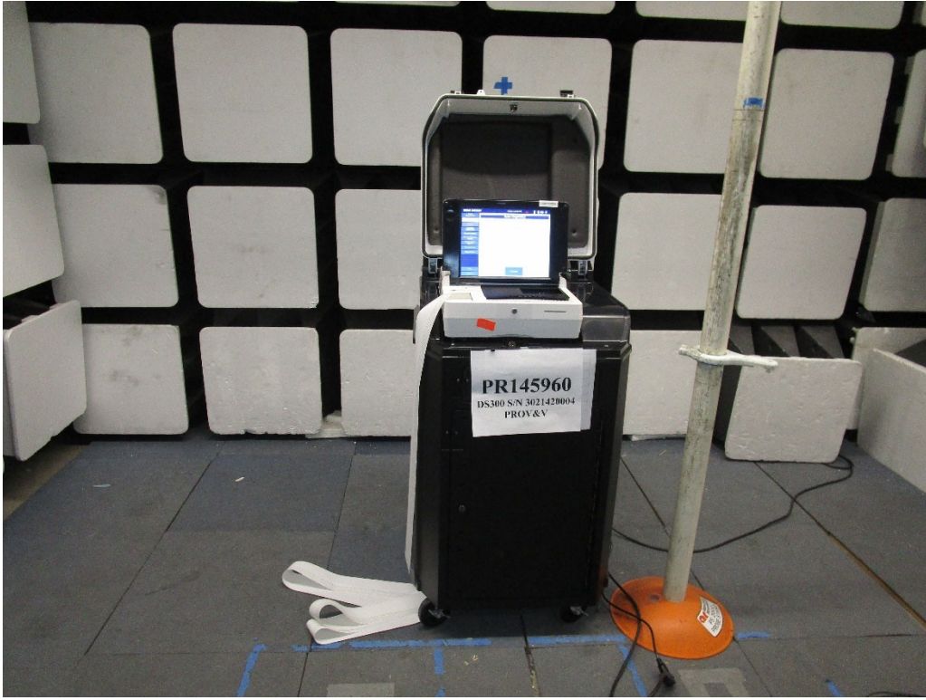
Radiated RF Immunity Test Setup – Front Side
