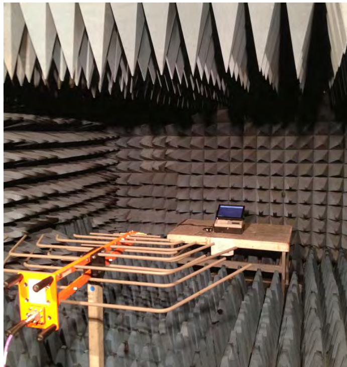
Photograph 9 Electromagnetic Susceptibility Test Set Up
