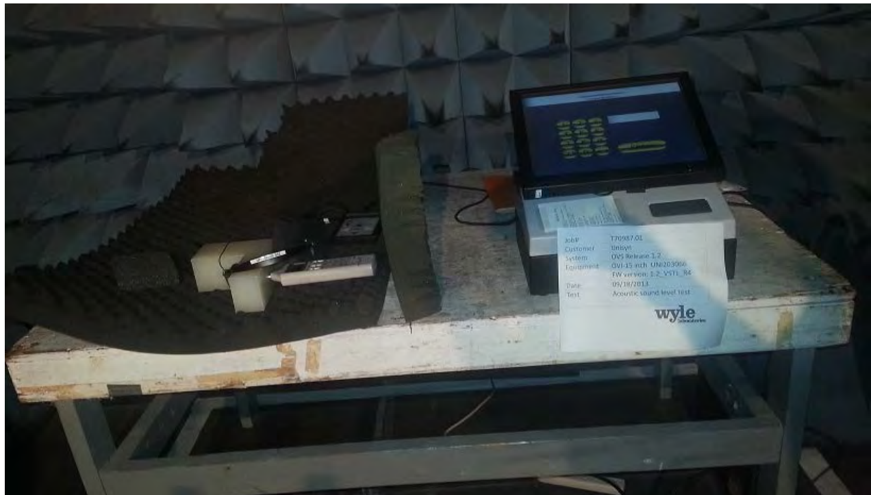
Photograph 11 Acoustic Sound Level Test Set Up
