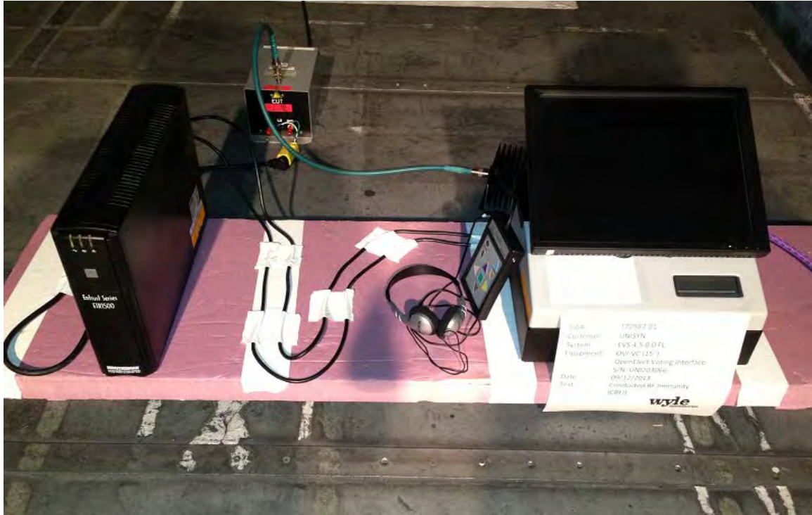
Photograph 6 Conducted RF Immunity Test Set Up
