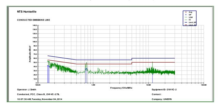
FCC Part 15, Conducted Emissions - Line - OVI-VC 2
