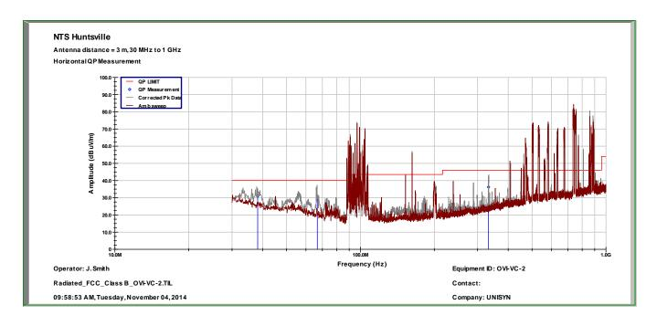
FCC Part 15, Radiated Emissions - Horizontal - OVI-VC 2
