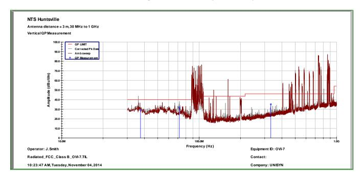
FCC Part 15, Radiated Emissions - Vertical - OVI-7
