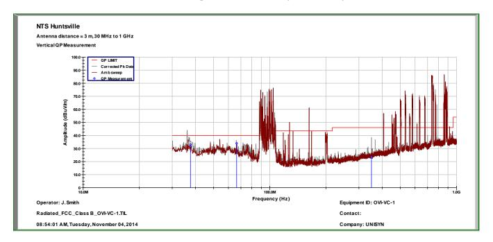
FCC Part 15, Radiated Emissions - Vertical - OVI-VC 1
