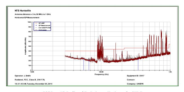
FCC Part 15, Radiated Emissions - Horizontal - OVI-7
