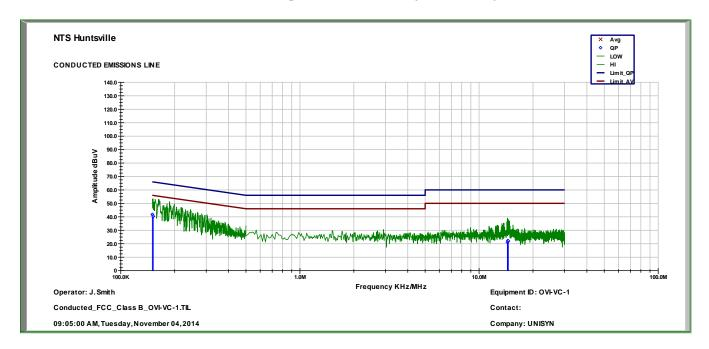
FCC Part 15, Conducted Emissions - Line - OVI-VC 1
