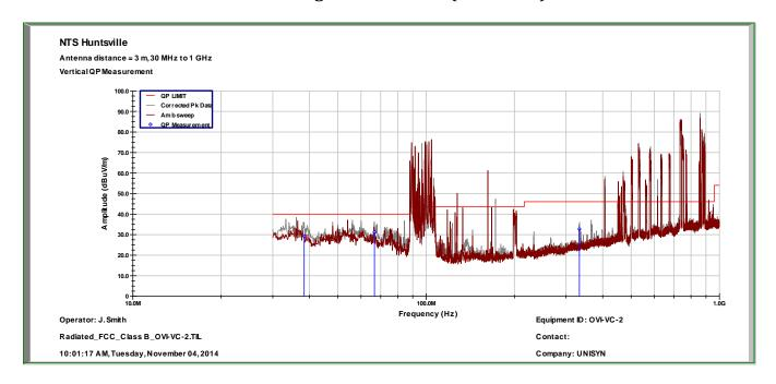
FCC Part 15, Radiated Emissions - Vertical - OVI-VC 2
