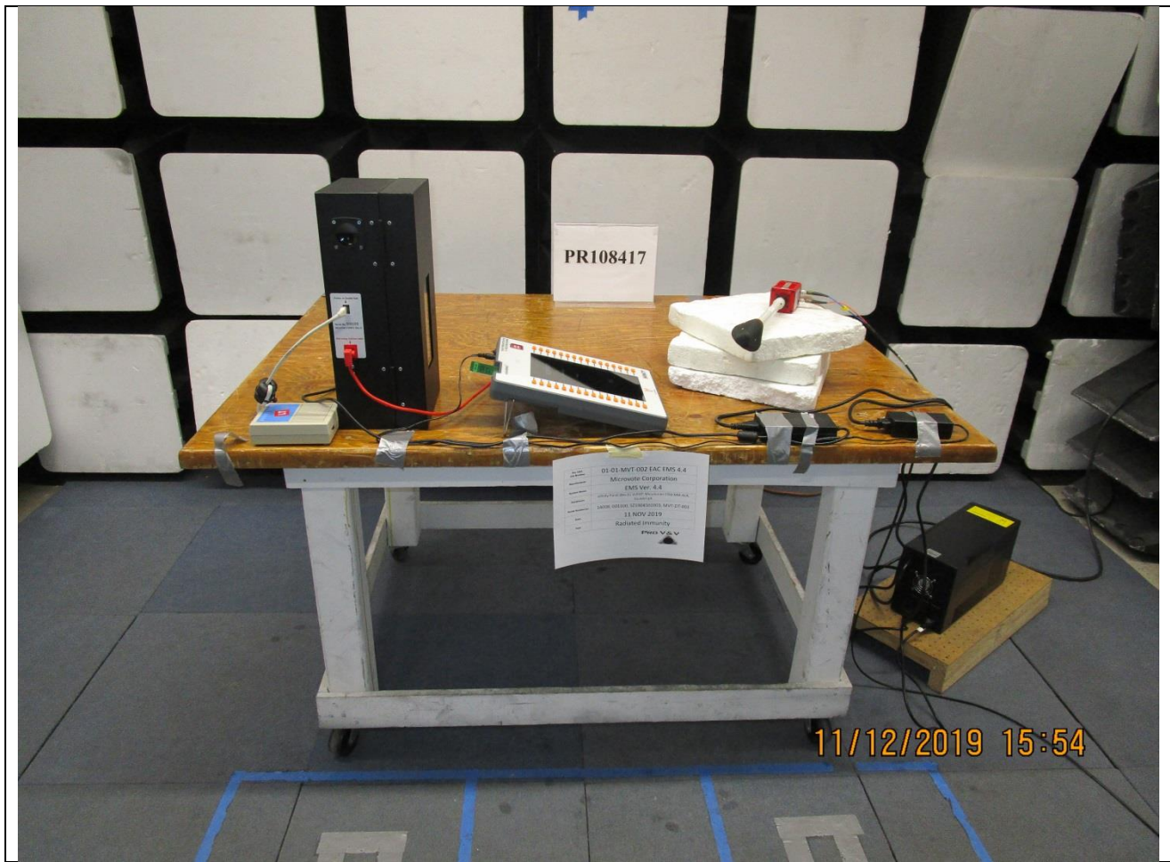
Figure B7. Radiated RF Immunity Test Setup – Left Side - UPS on floor.
