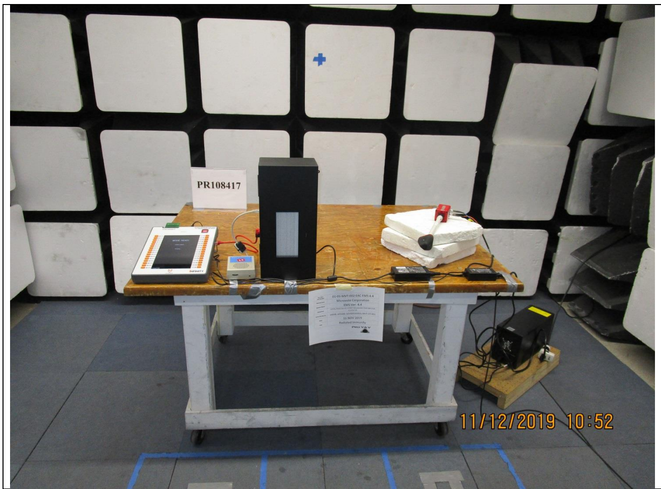
Figure B4. Radiated RF Immunity Test Setup – Front Side - UPS on floor.
