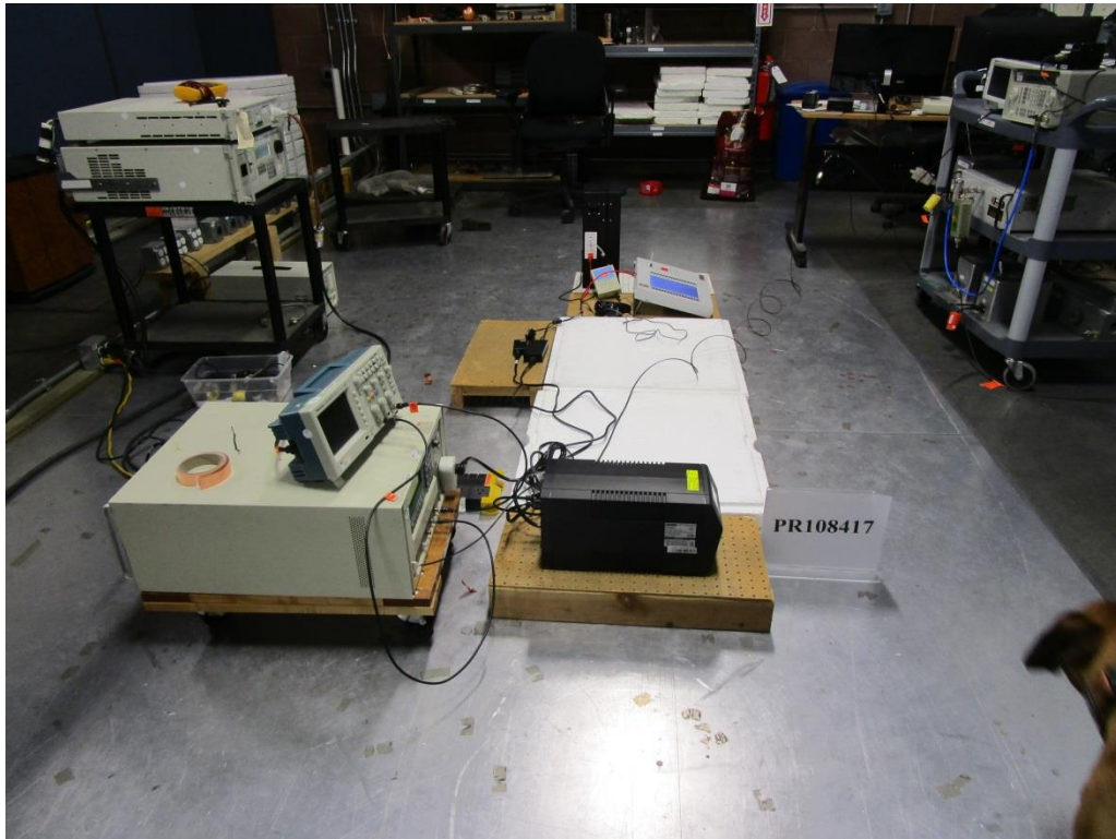
Figure D1. Surge Immunity Test Setup.
