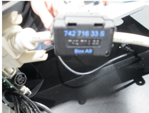
Wurth ferrite 742-716-33 s to the data line
