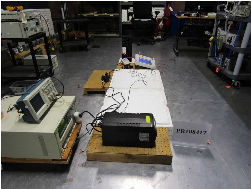
Figure C1. Electrical Fast Transient Test Setup.
