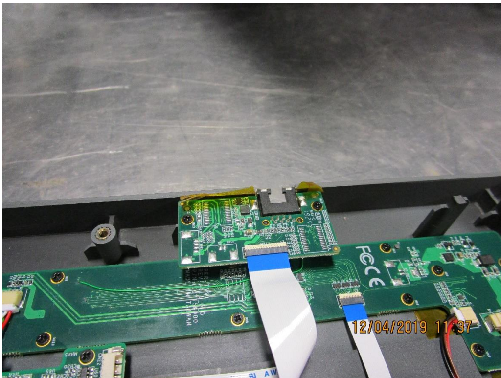
Kapton tape fix on Ethernet board.
