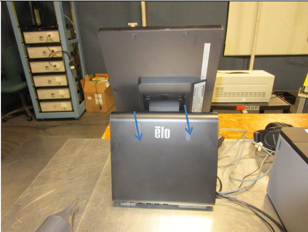
Figure A12. Electrostatic Discharge Test Setup.
