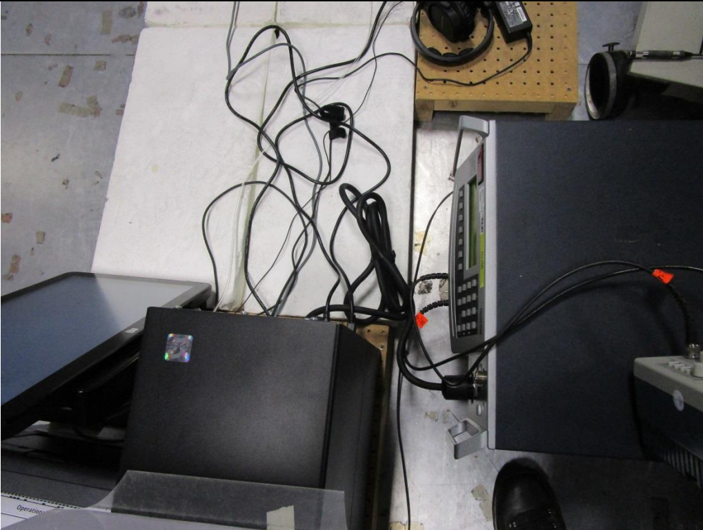
Figure C2. Electrical Fast Transient Test Setup – AC Mains.
