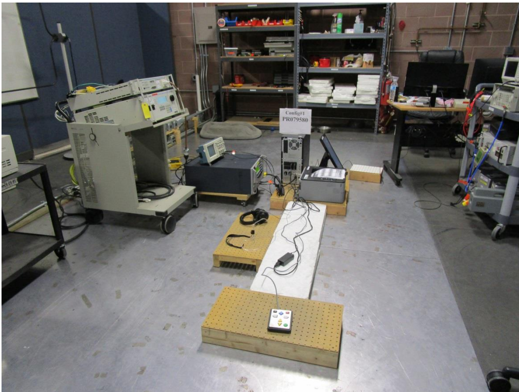
Figure D1. Surge Immunity Test Setup.
