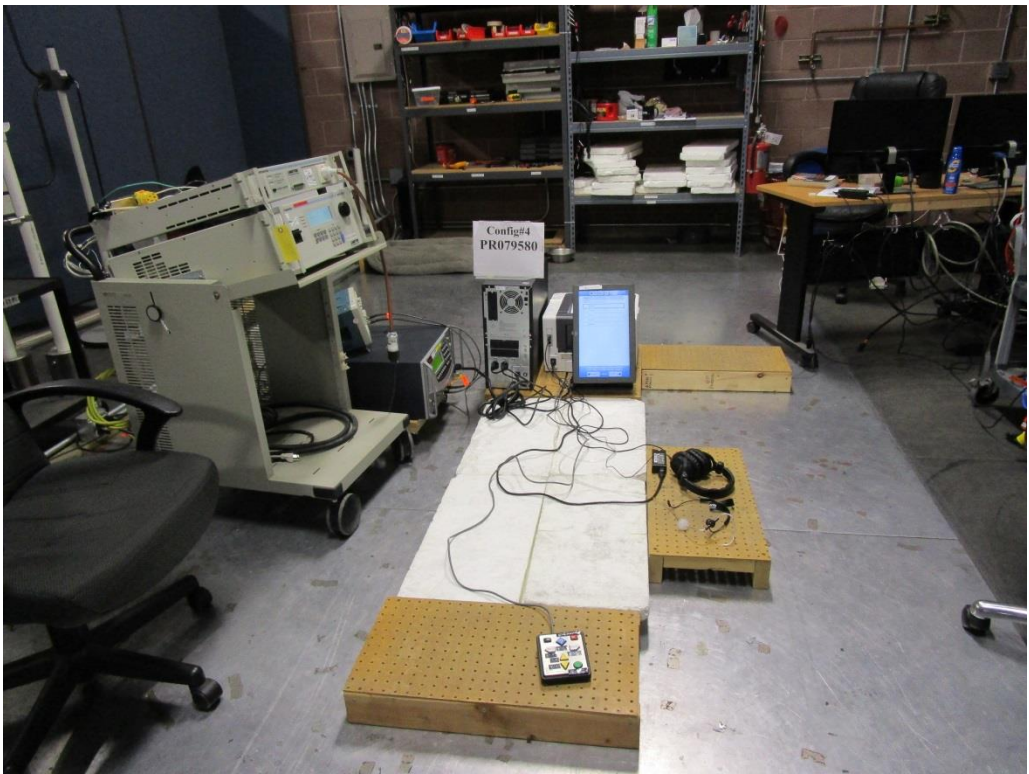
Figure D1. Surge Immunity Test Setup.
