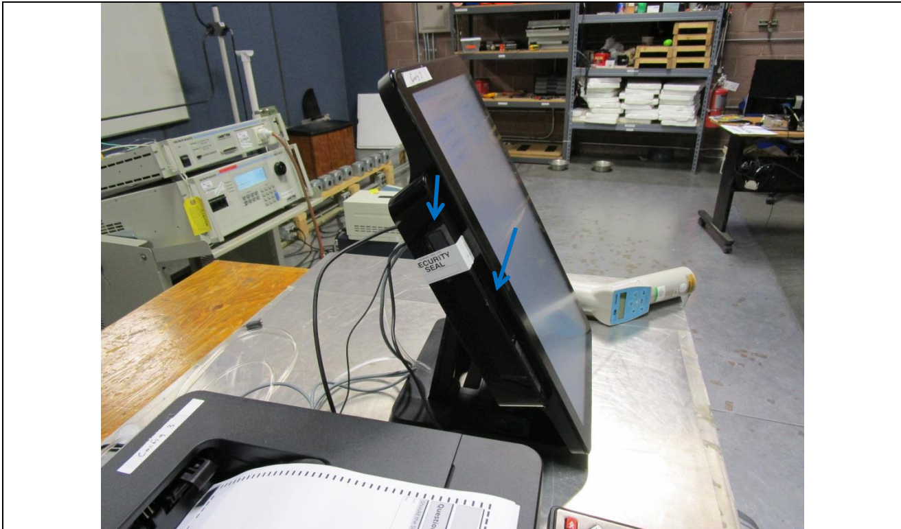
Figure A11. Electrostatic Discharge Test Setup.
