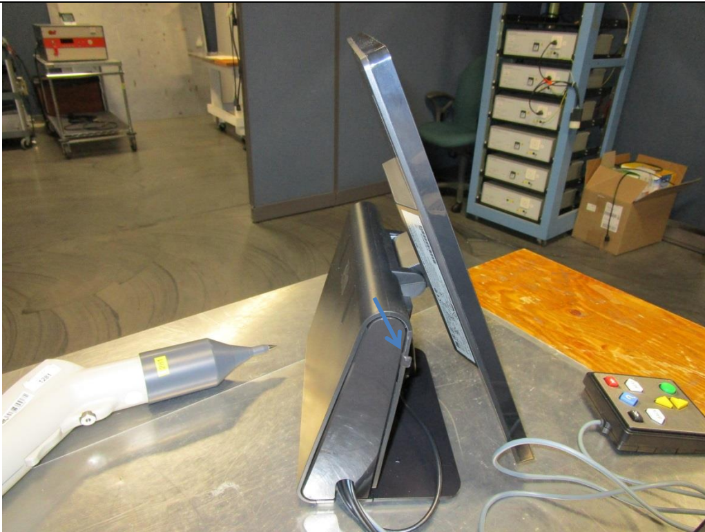
Figure A13. Electrostatic Discharge Test Setup.
