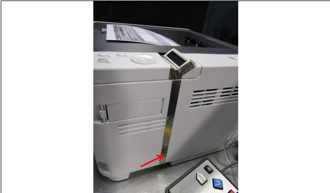
Figure A7. Electrostatic Discharge Test Setup.
