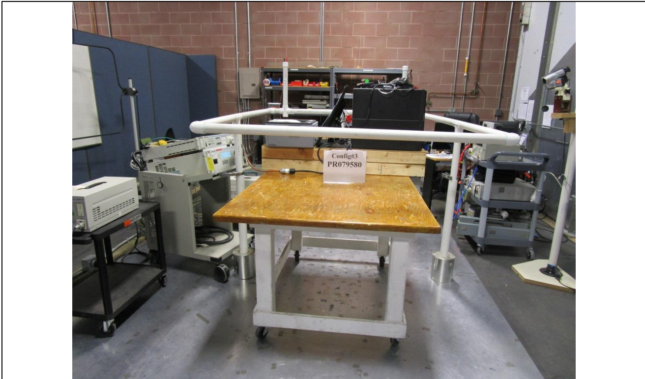
Figure F3. Power Frequency H-field Immunity Test Setup Z axis.
