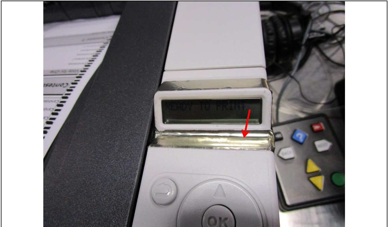
Figure A6. Electrostatic Discharge Test Setup.
