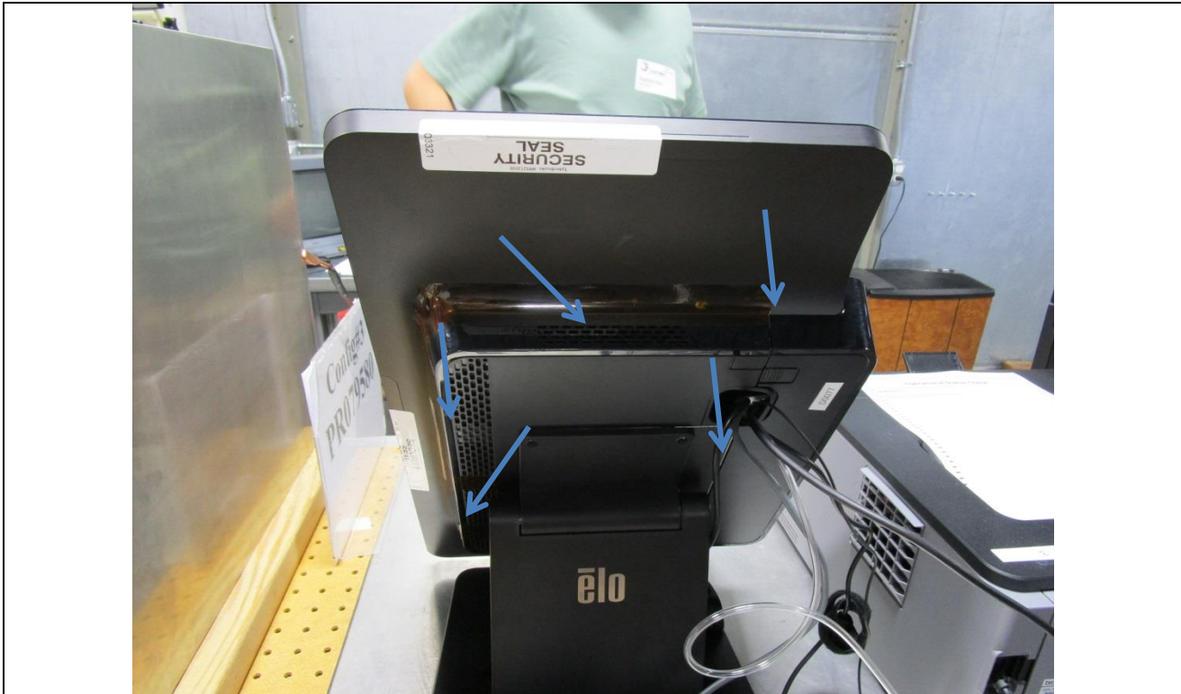
Figure A16. Electrostatic Discharge Test Setup.
