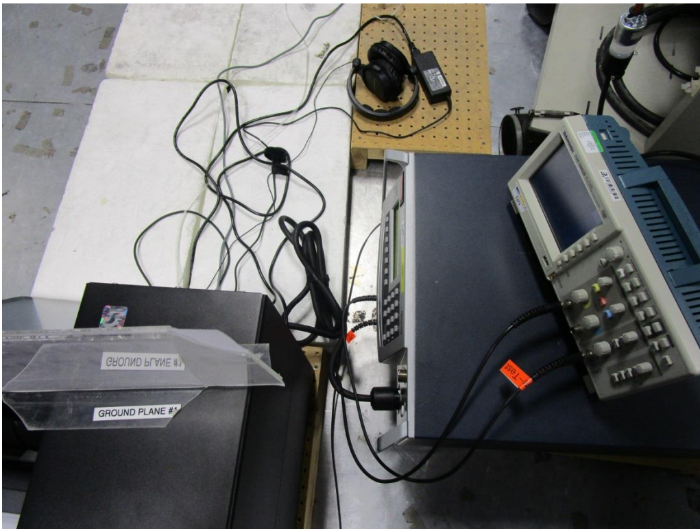
Figure G2. Voltage Dips and Interruptions Test Setup.
