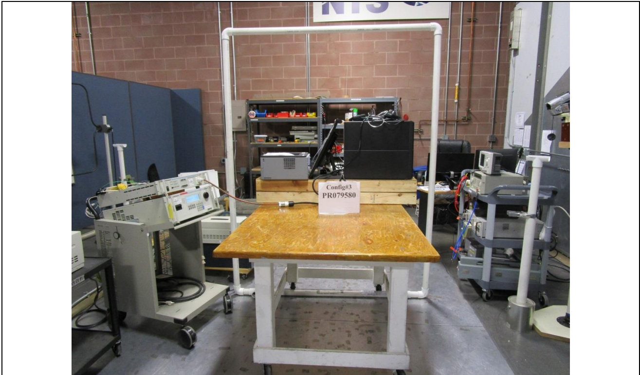
Figure F2. Power Frequency H-field Immunity Test Setup Y axis.
