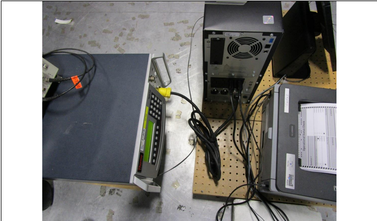
Figure C2. Electrical Fast Transient Test Setup – AC Mains.
