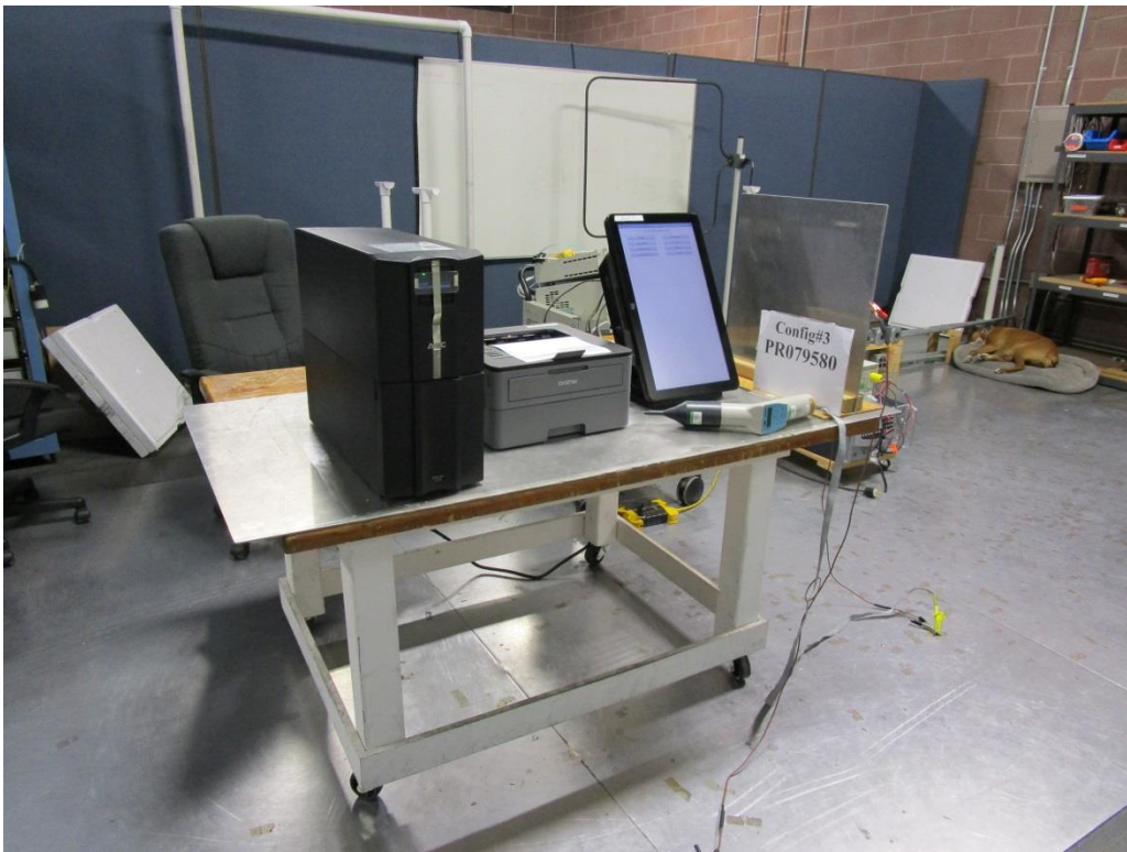
Figure A1. Electrostatic Discharge Test Setup.
