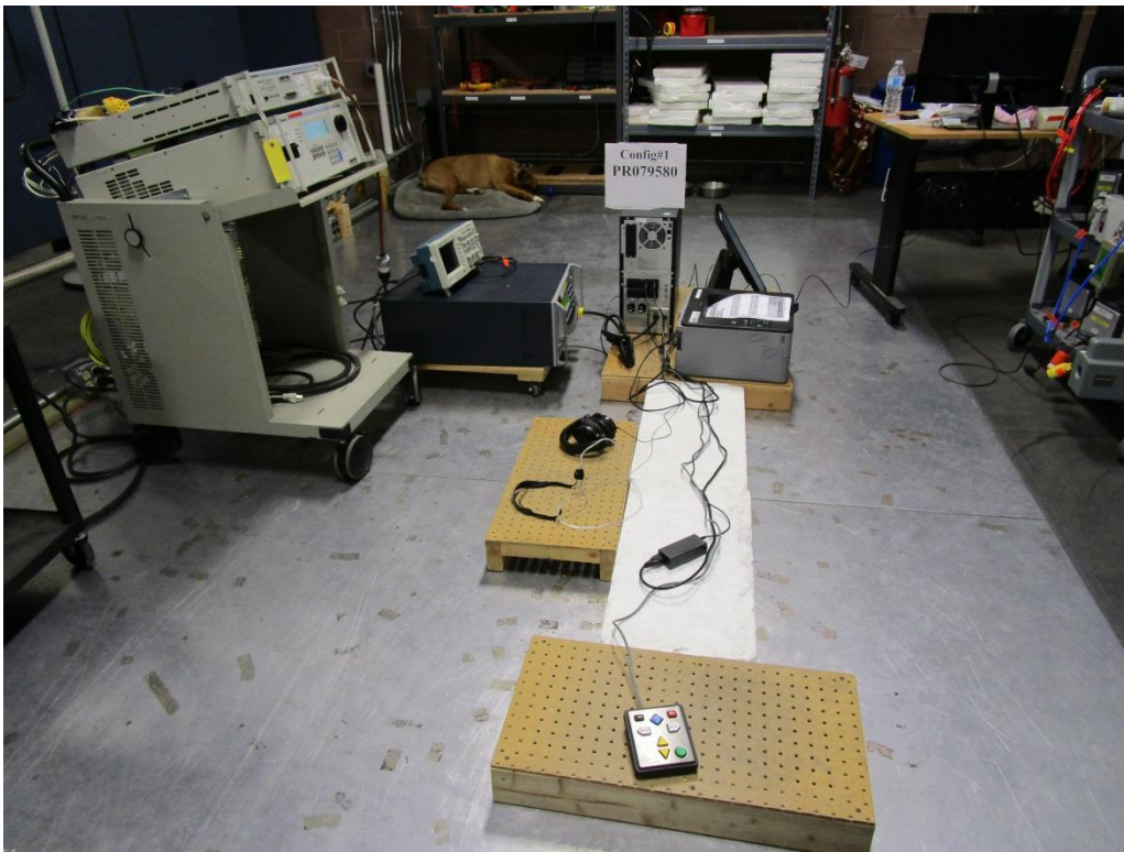
Figure C1. Electrical Fast Transient Test Setup.
