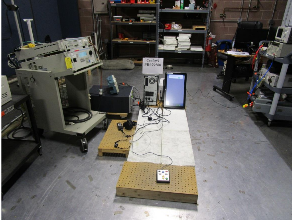
Figure G1. Voltage Dips and Interruptions Test Setup.
