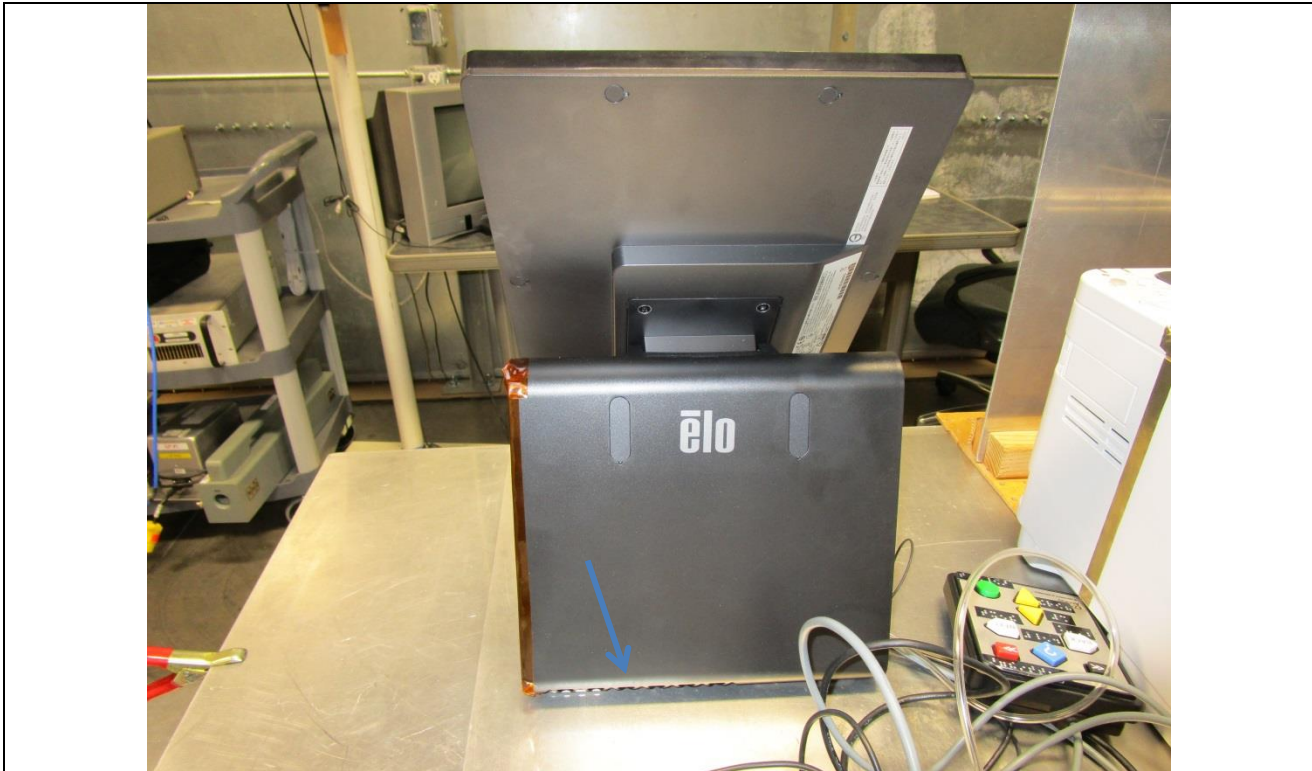
Figure A8. Electrostatic Discharge Test Setup.
