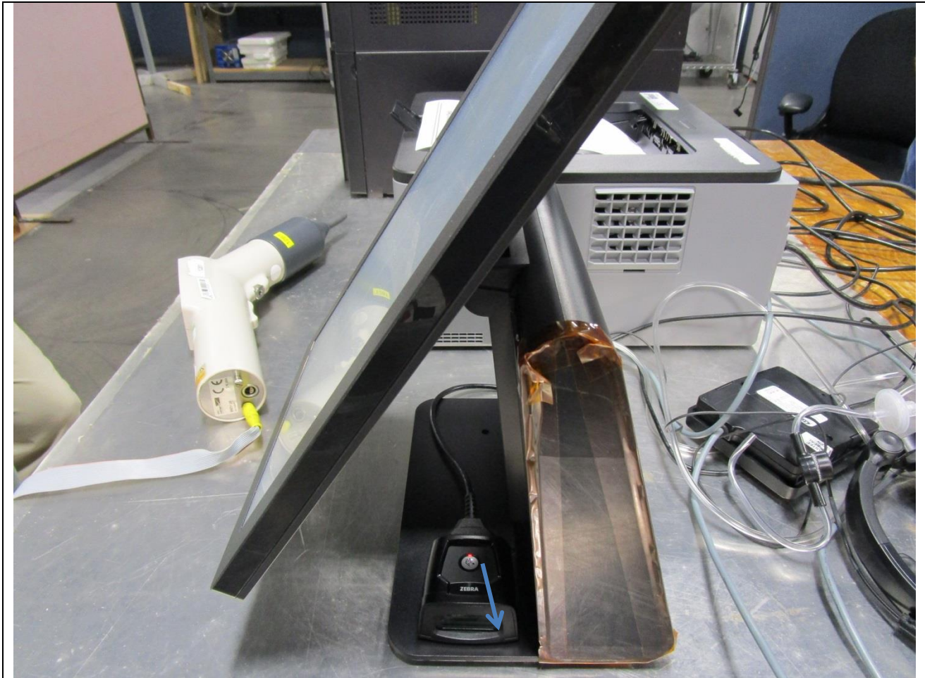
Figure A11. Electrostatic Discharge Test Setup.
