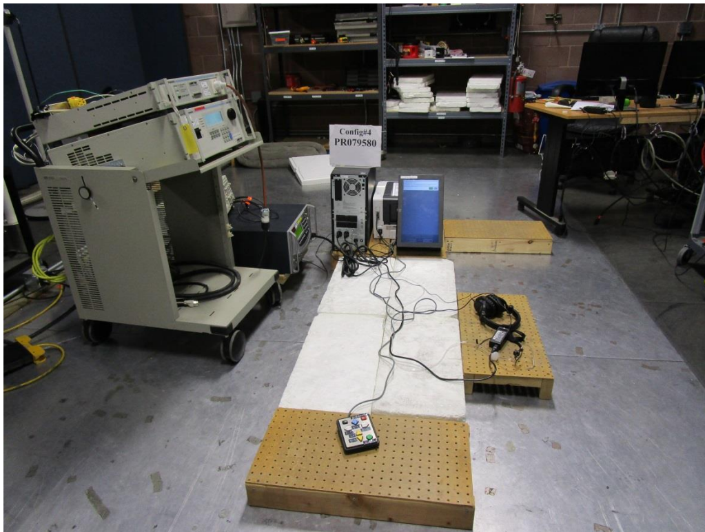
Figure C1. Electrical Fast Transient Test Setup.
