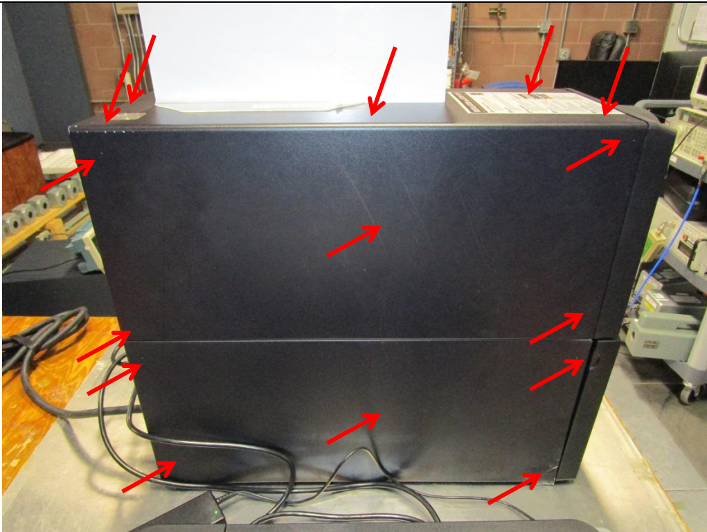
Figure A5. Electrostatic Discharge Test Setup.
