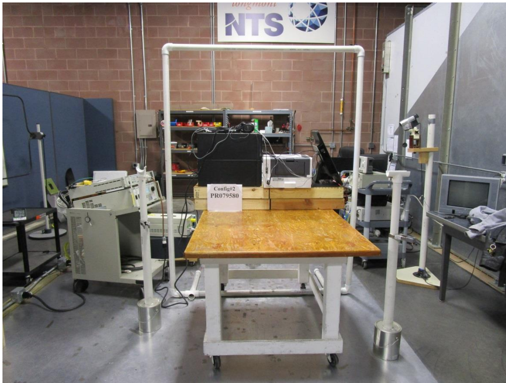
Figure F1. Power Frequency H-field Immunity Test Setup X axis.
