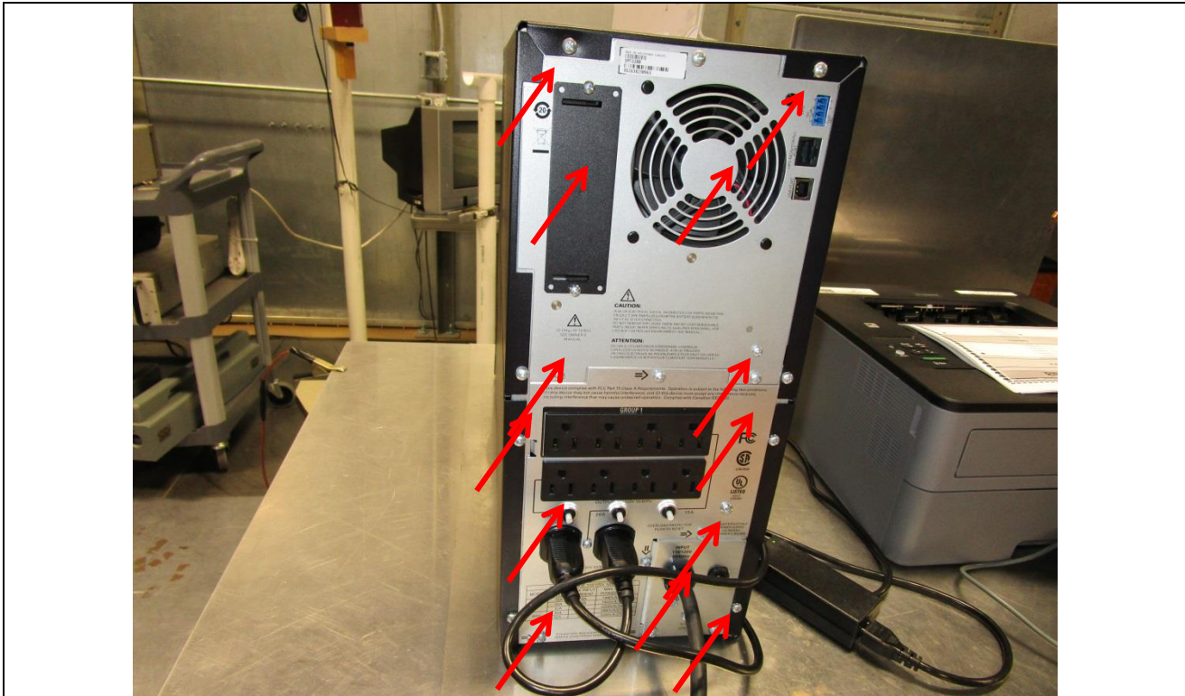
Figure A4. Electrostatic Discharge Test Setup.
