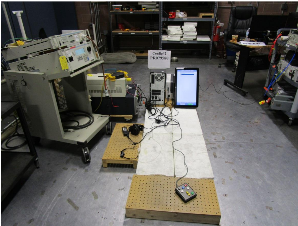
Figure C1. Electrical Fast Transient Test Setup.
