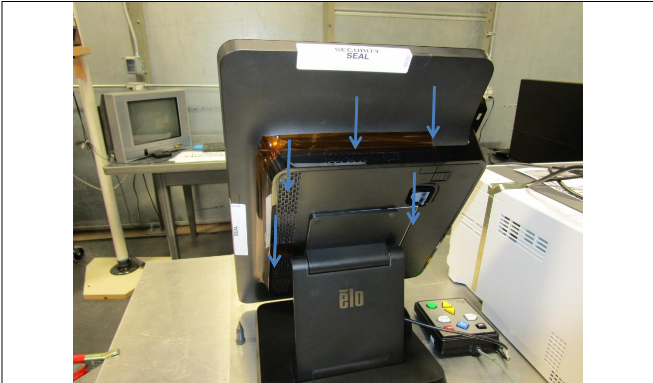
Figure A12. Electrostatic Discharge Test Setup.
