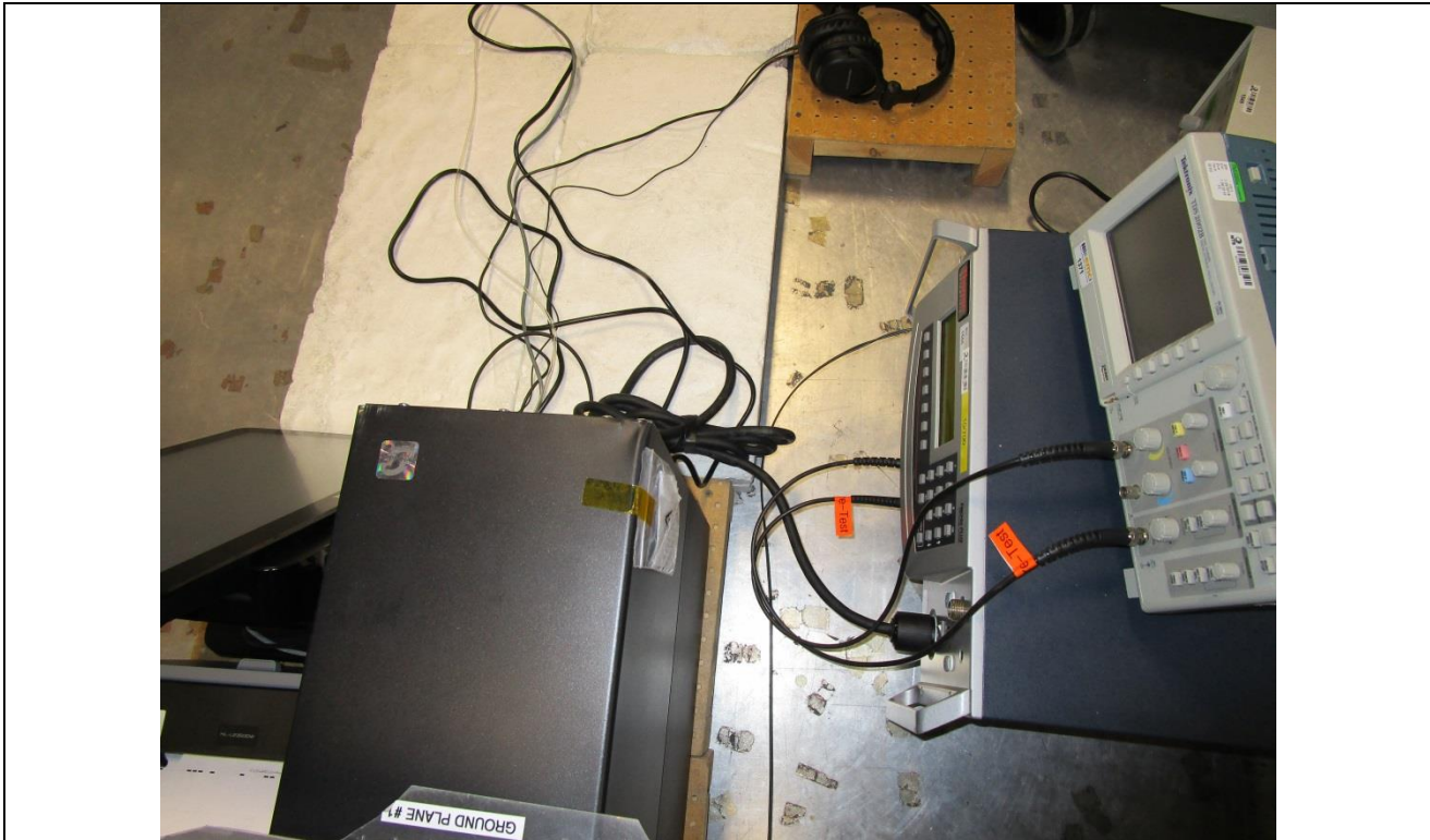
Figure D2. Surge Immunity Test Setup – AC Mains.
