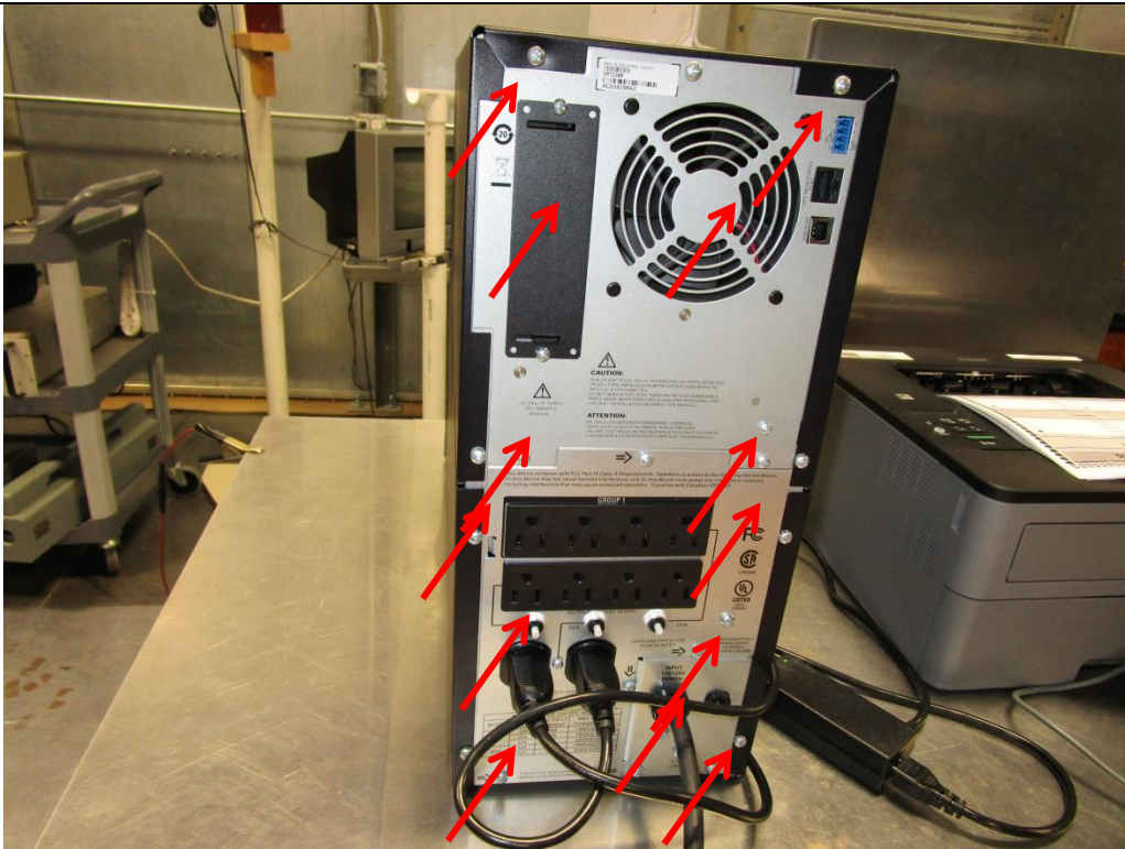
Figure A4. Electrostatic Discharge Test Setup.
