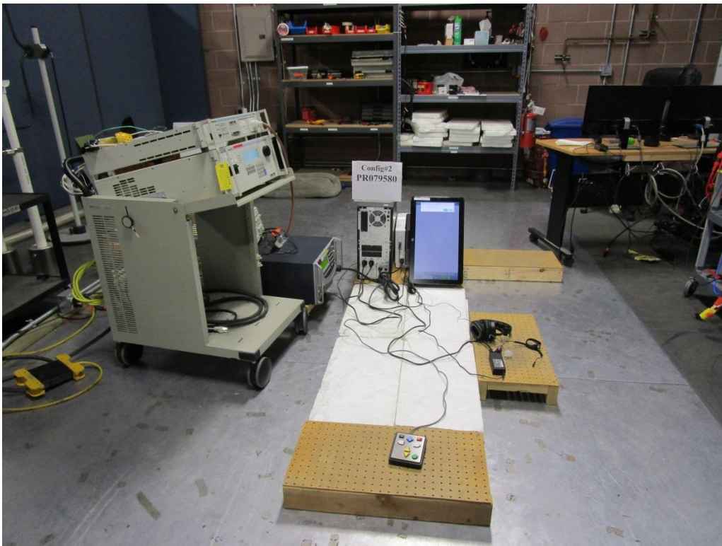
Figure D1. Surge Immunity Test Setup.
