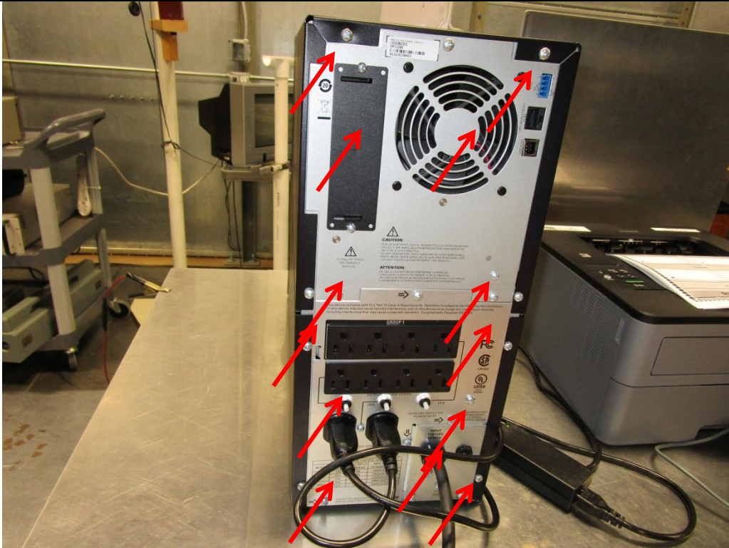
Figure A4. Electrostatic Discharge Test Setup.
