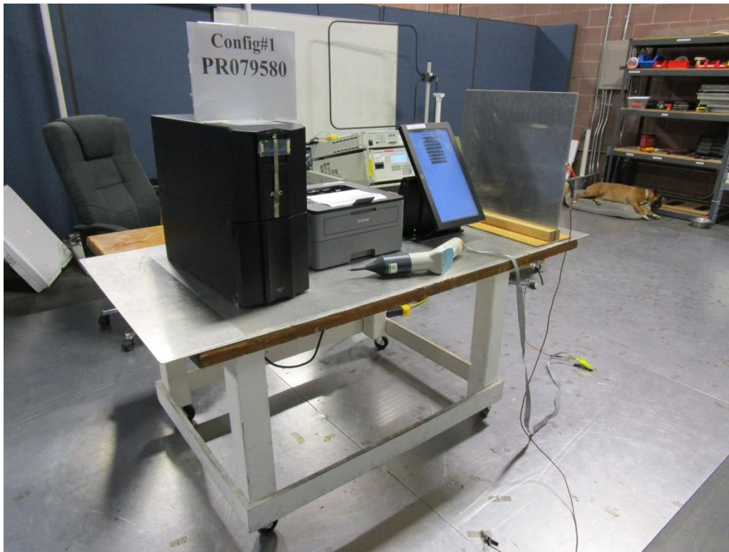
Figure A1. Electrostatic Discharge Test Setup.
