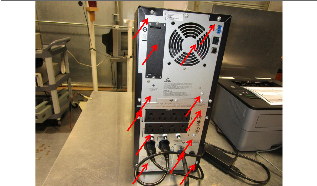
Figure A4. Electrostatic Discharge Test Setup.
