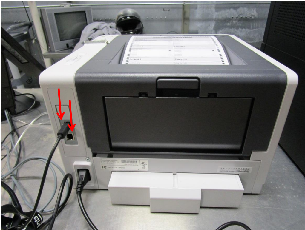
Figure A12. Electrostatic Discharge Test Setup.
