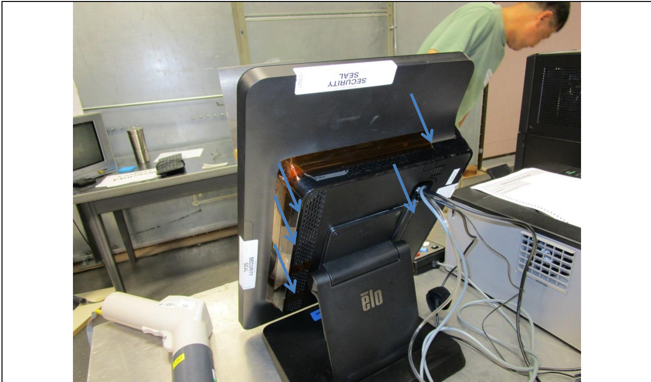
Figure A12. Electrostatic Discharge Test Setup.
