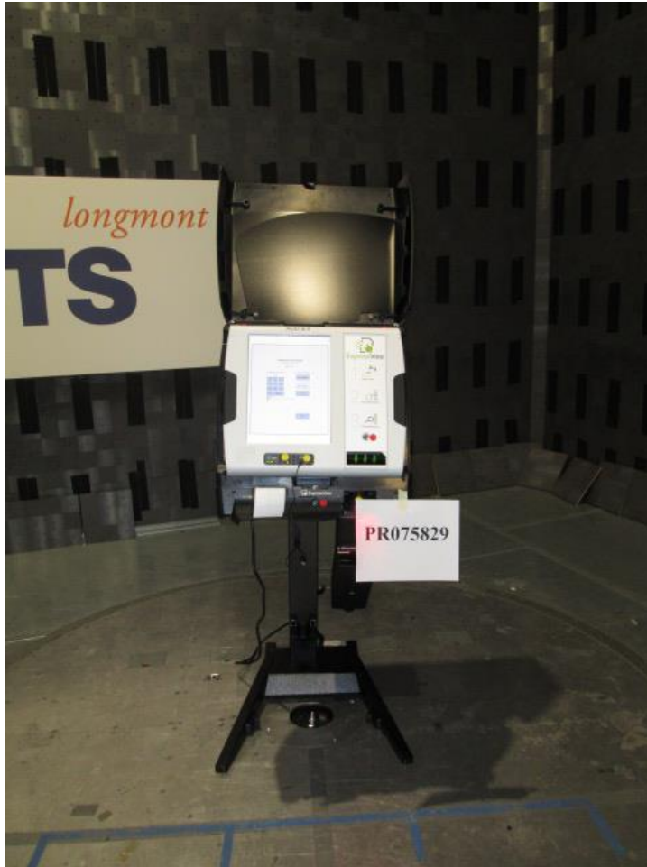
Figure A3: Radiated Emissions Test Setup – Front Side
