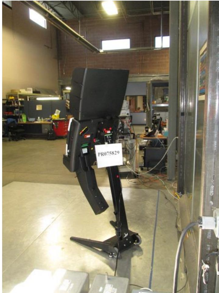
Figure B5: Conducted Emissions Test Setup – Back Side
