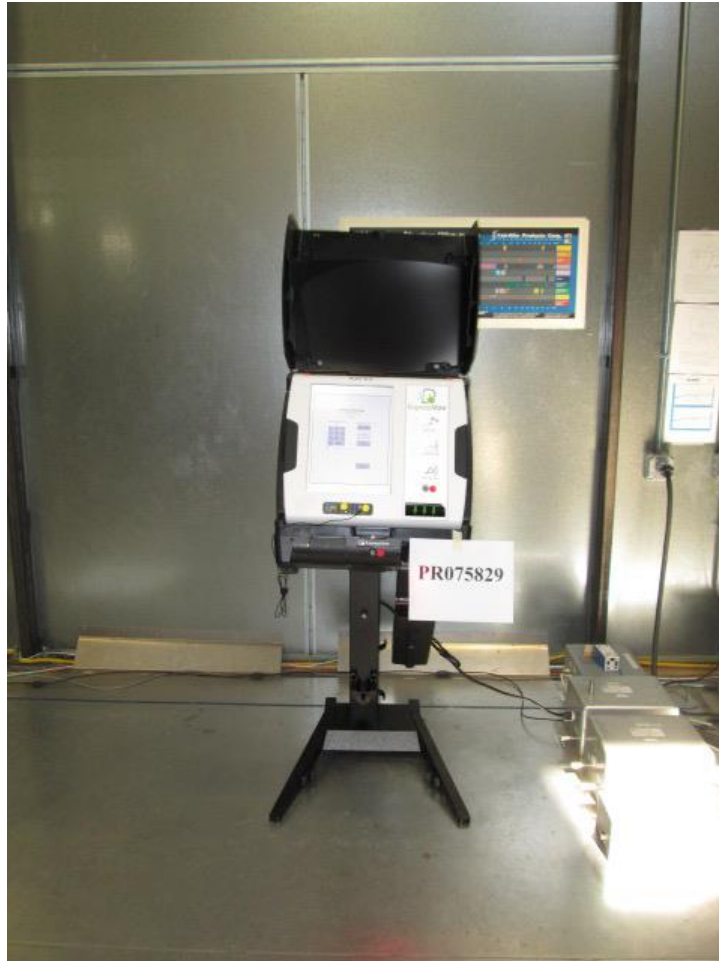
Figure B3: Conducted Emissions Test Setup – Front Side
