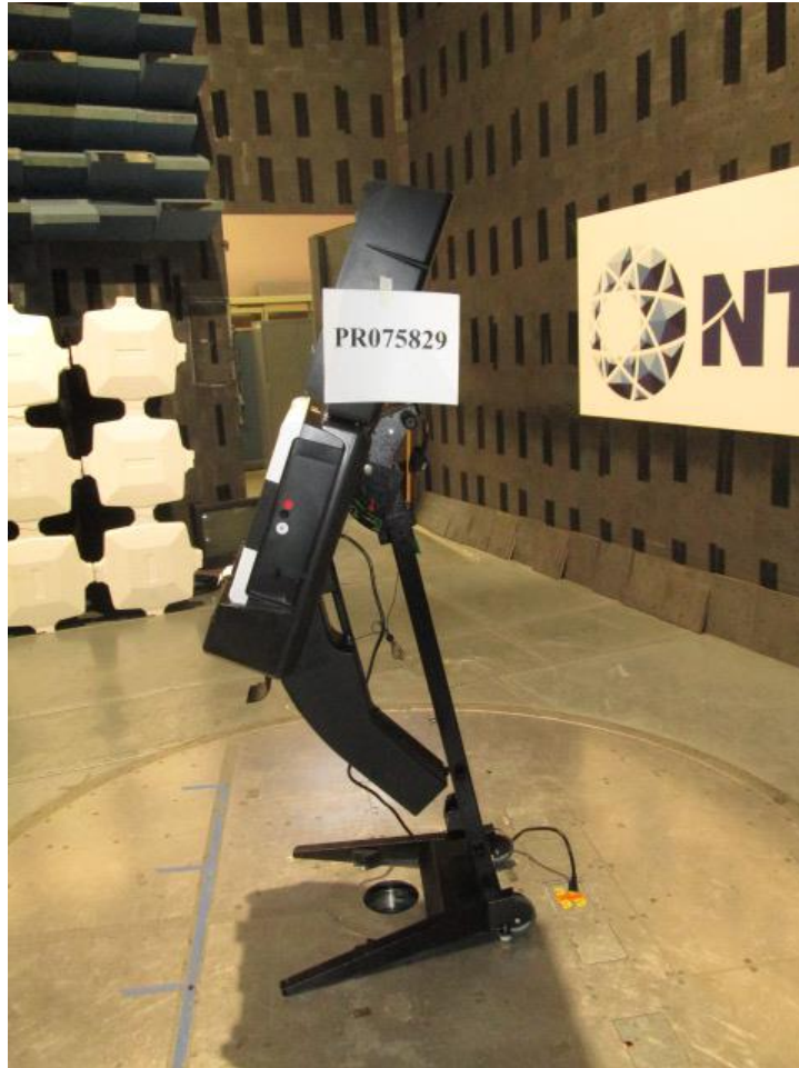
Figure A4: Radiated Emissions Test Setup – Right Side
