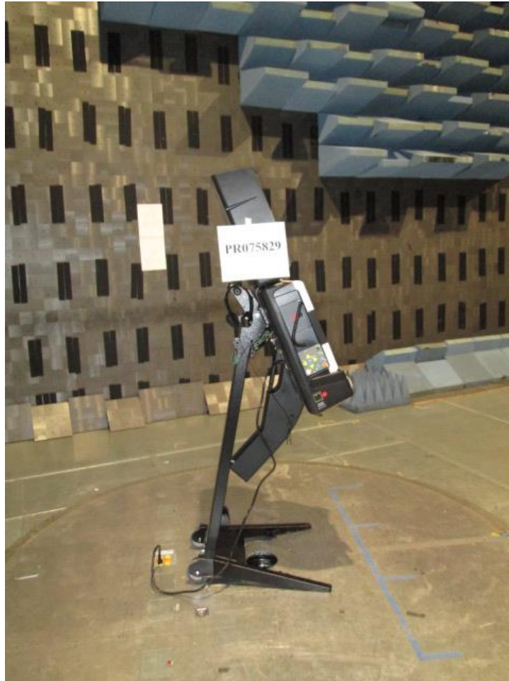
Figure A6: Radiated Emissions Test Setup – Left Side
