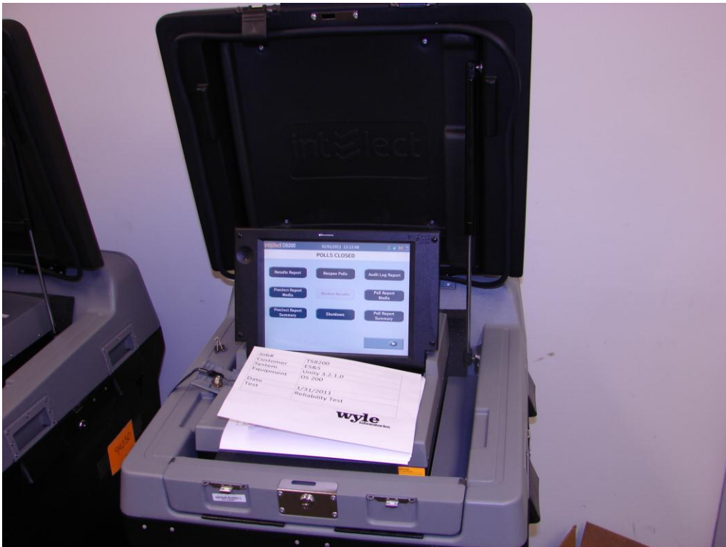
Photograph 4: ES&S Unity 3.2.1.0 Reliability Test Setup
