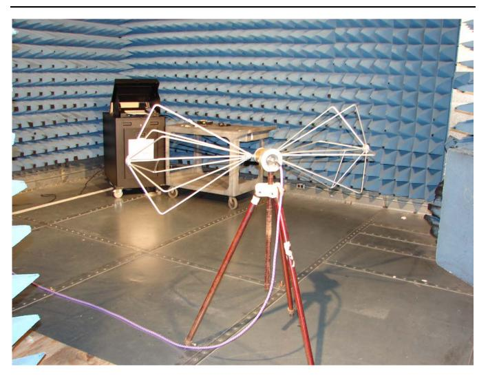
Photograph 2 ICP Electromagnetic Radiation Test Setup
