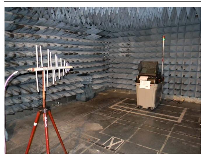
Photograph 1 ICE Electromagnetic Radiation Test Setup
