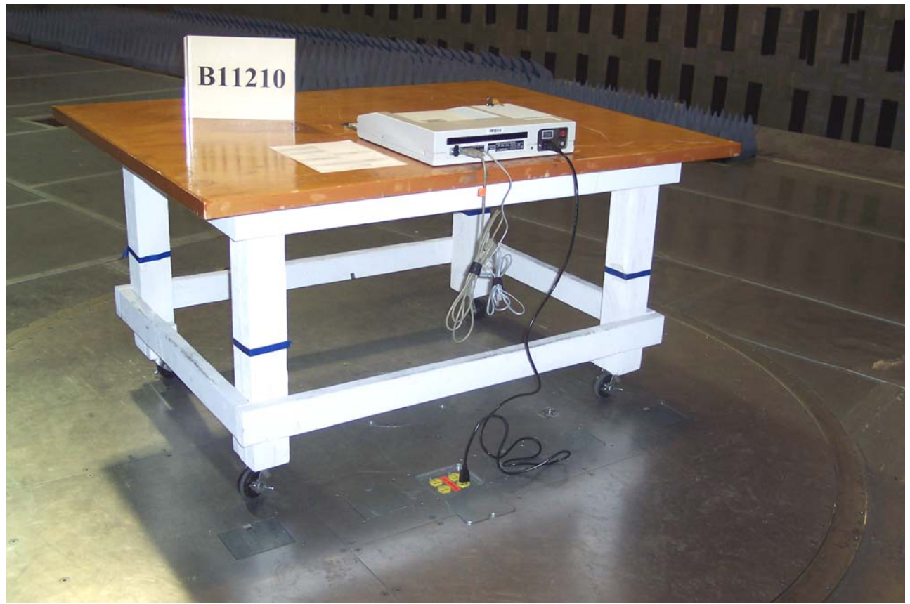
Figure A4: Radiated Emissions Test Setup – Back
