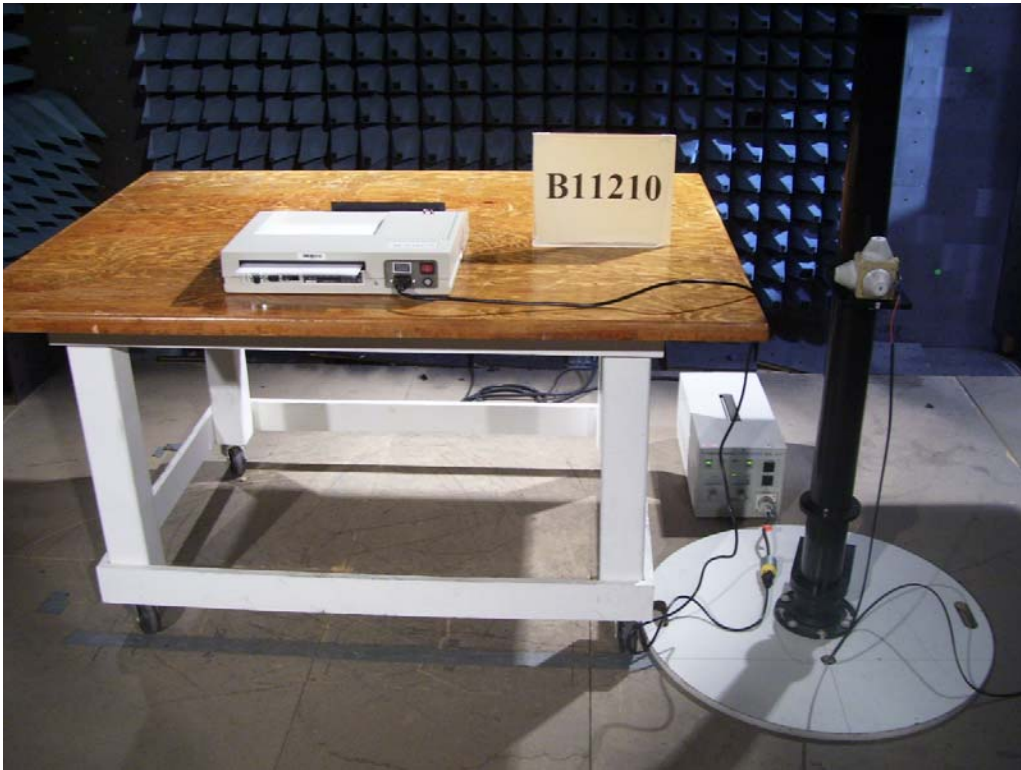
Figure C3. Radiated RF Immunity Test Setup – Back Side.
