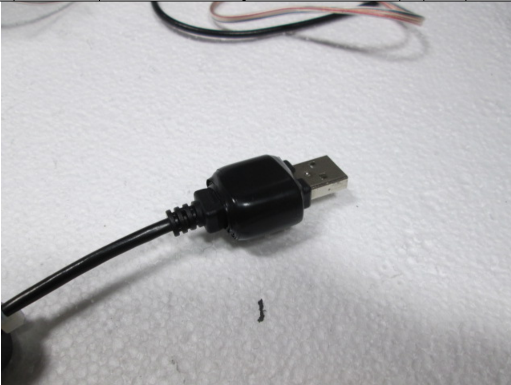
Modification to UUT, added electrical tape to USB cable connector.
