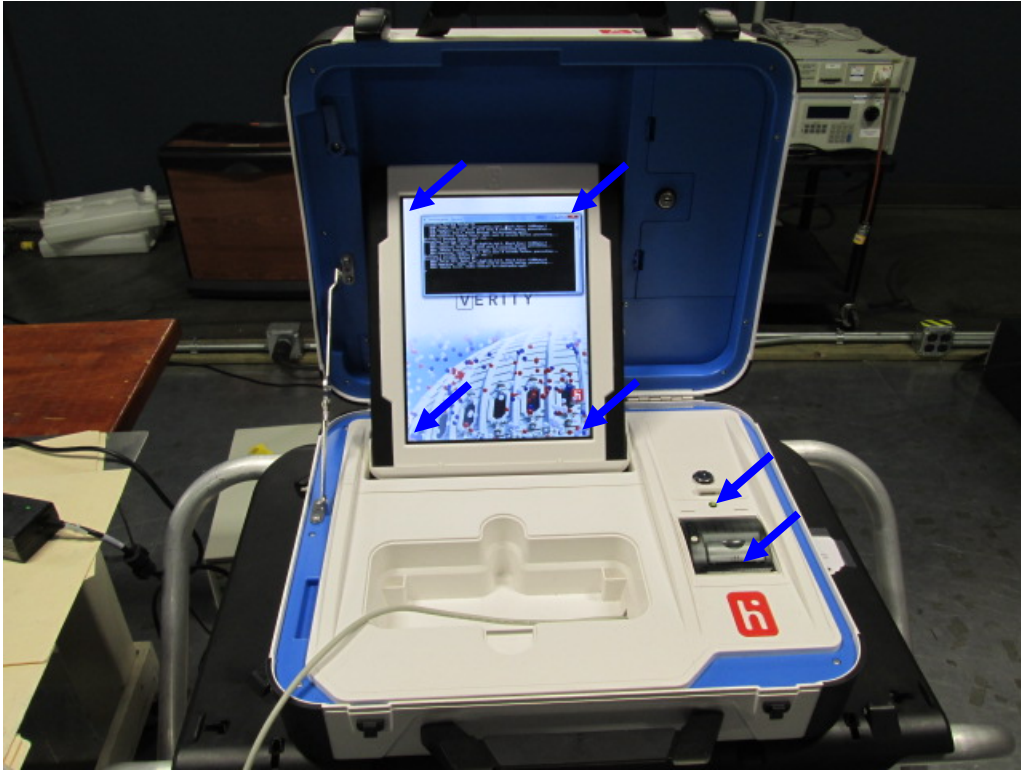
Figure A5. Electrostatic Discharge Test Setup.
