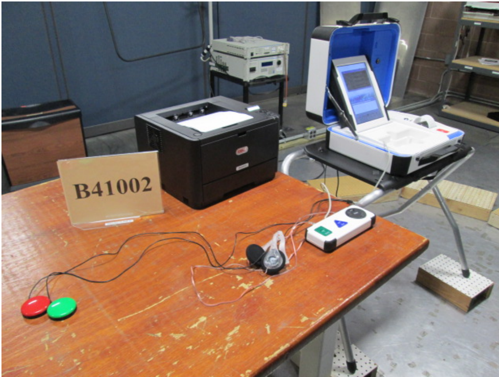
Figure D1. Surge Immunity Test Setup
