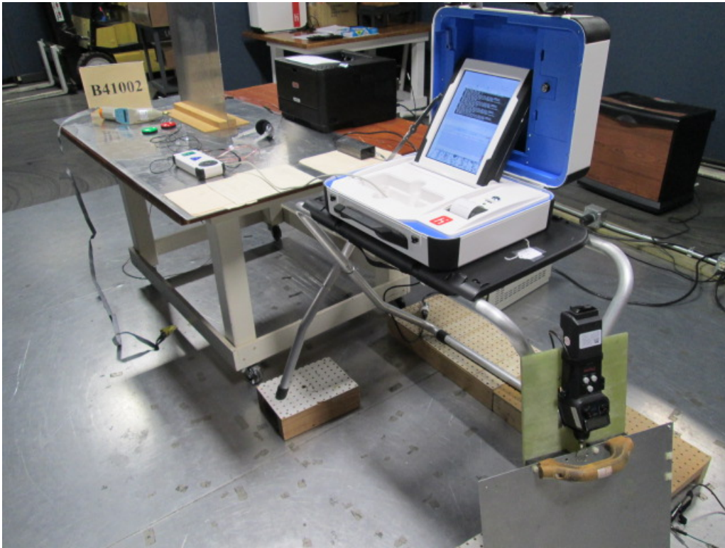
Figure A1. Electrostatic Discharge Test Setup.
