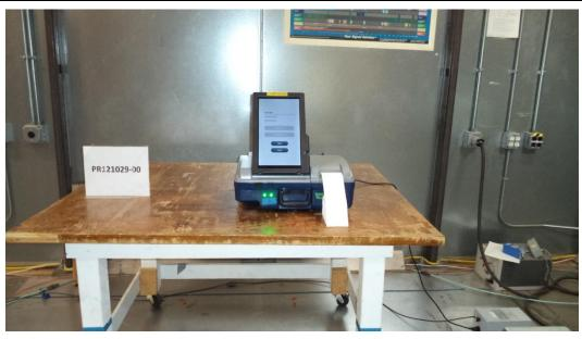
Figure A1. Conducted Emissions Test Setup.
