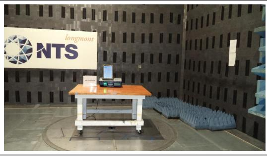
Figure A1. Radiated Emissions Test Setup (Front).
