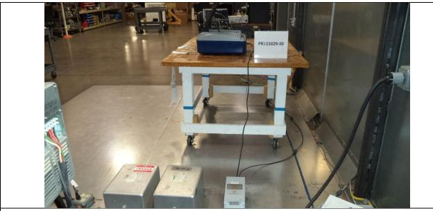
Figure A3. Conducted Emissions Test Setup.
